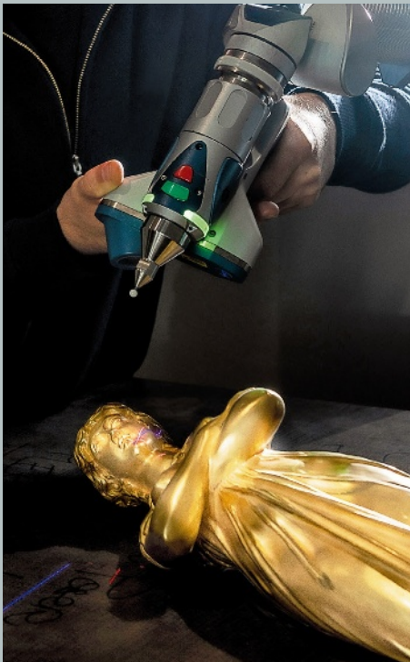
Digital scans Two lasers overlap on the object to scan, modeling it via a multitude of points.
